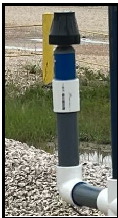
Figure 11. Communication Antenna. Sends local measurements to Earthview cloud servers.
