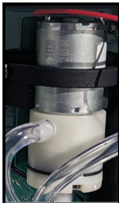
Figure 16: Pump: pulls outside air into sample chamber.
